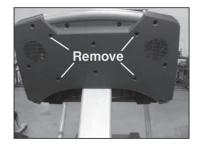
Remove the four screws from the tread display as shown.
