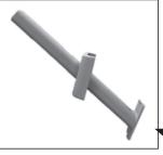
Slide the top mounting plate on the neck and align the top plate notch with the neck base notch.
