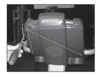
Remove the four screws from the display. (Screws are no longer needed)
